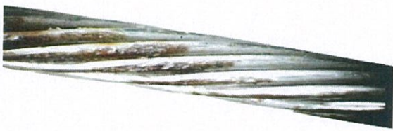
Rust or Corrosion
