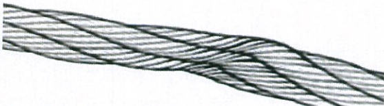
Crushed or Flattened
